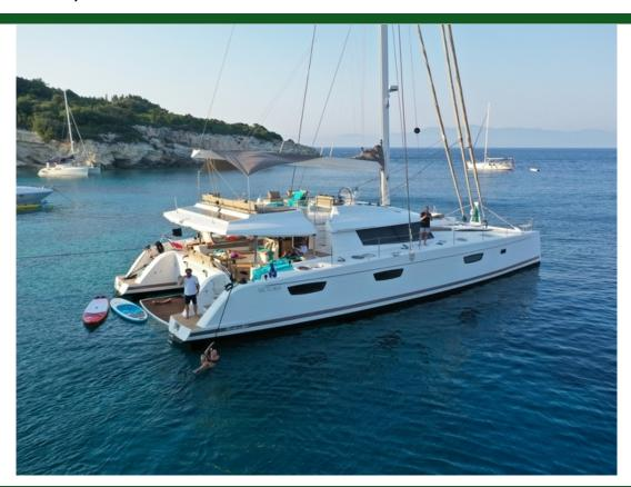
种类现代游艇类型帆船船身类型双体船载客量21.7m (72 ')船宽9.5m (32')吃水1.9m (7')船身材料玻璃钢
