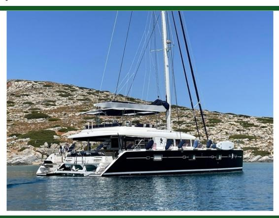
种类现代游艇类型帆船船身类型双体船载客量19m (62.0 ' )船宽10.0m (33')吃水1.5m (5')船身材料玻璃钢
