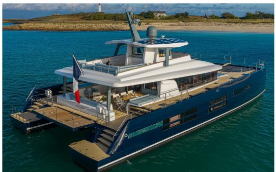
Type Modern Propulsion Power Hull Catamaran Length 23.7m (78') Beam 11.2m (37') 1.2m (4') Draft **Hull Material** Aluminium
