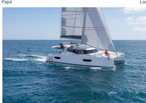
Modern Type Propulsion Sail Hull Catamaran Length 13.5m (45') Beam 7.5m (25') Draft 1.2m (4') **Hull Material** Fiberglass Engine 2 / Nanni /
