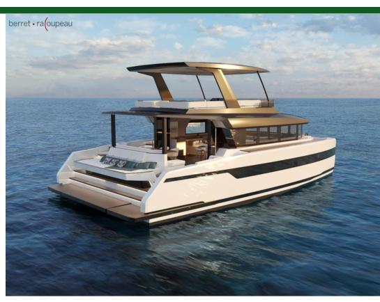
Type Modern Propulsion Power Catamaran Hull 15.0m (50') Length Beam 7.5m (25') Draft 0.9m (3') **Hull Material Fiberglass** 2 / Torqeedo / Engine
