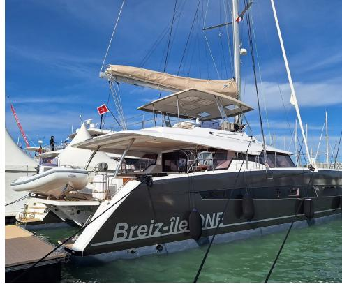
Type Modern Propulsion Sail Hull Catamaran Length 19.5m (64') Beam 9.8m (33') Draft 1.7m (6') **Hull Material** Fiberglass
