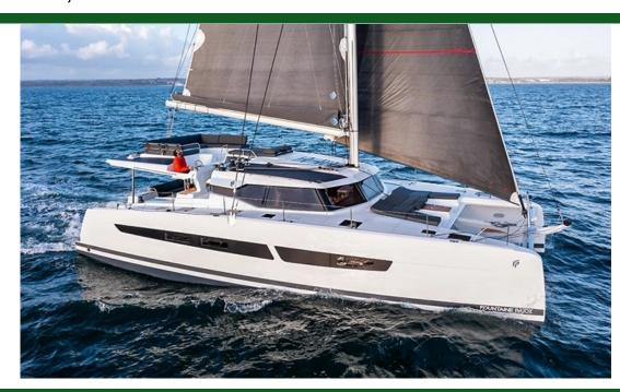
Type Modern Propulsion Sail Hull Catamaran 15.5m (51') Length 8.1m (27') Beam Draft 1.3m (5') **Hull Material** Fiberglass Engine 2 / Volvo / D2
