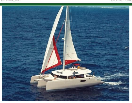
Type Modern Propulsion Sail Hull Trimaran Length 15.6m (52') Beam 8.9m (30') Draft 1.8m (6') Fiberglass **Hull Material** 1 / Volvo / D2 Engine
