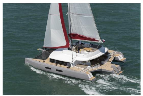
Type Modern Propulsion Sail Hull Trimaran Length 19.8m (65') Beam 12.0m (40') Draft 1.8m (6') **Hull Material Fiberglass** Engine 1 / Volvo / Engine HP 150
