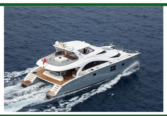
Type Modern Propulsion Power Hull Catamaran Length 21.4m (71') Beam 9.3m (31') Draft 1.2m (4') Composite **Hull Material** Engine 2 / Man / R6 Engine HP 800
