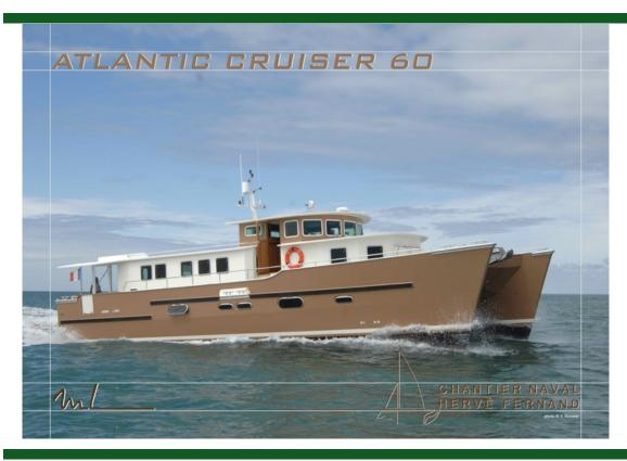
Classic Type Propulsion Power Hull Catamaran Length 18.6m (62') 7.7m (26') Beam 1.2m (4') Draft **Hull Material** Composite **Engine** 2 / Cummins /
