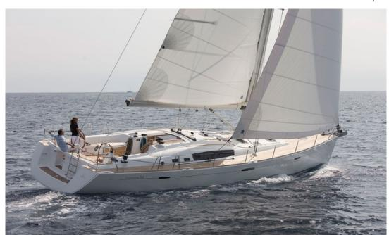
Type Modern Propulsion Sail Hull Mono Length 16.7m (55') 4.9m (17') Beam Draft 1.8m (6') **Hull Material Fiberglass Engine** 1 / Yanmar /
