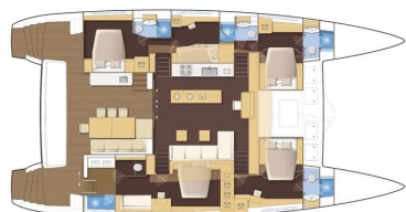
Cabine centrale, 5 cabines / Central galley, 5 cabin version
