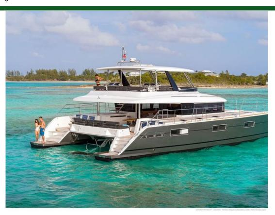
Type Modern Propulsion Power Hull Catamaran Length 20m (64.0') 10m (32.1') Beam Draft 2m (3.8') **Hull Material Fiberglass Engine** 2 / Volvo / D4-300
