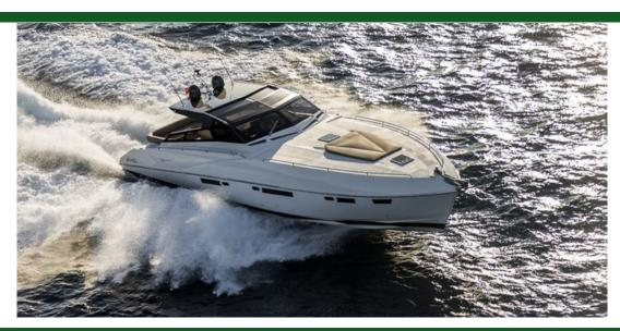
种类现代游艇类型机动游艇船身类型单体船载客量17.9m (59 ' )船宽5.1m (17')吃水1.3m (5')船身材料玻璃钢
