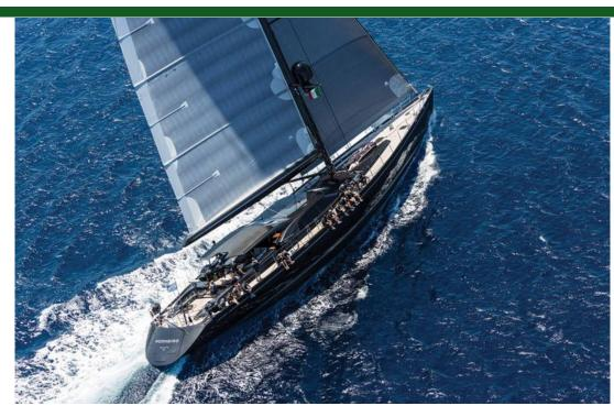
种类现代游艇类型帆船船身类型单体船载客量37.1m (122 ' )船宽8.3m (28')吃水4.1m (14')船身材料铝
