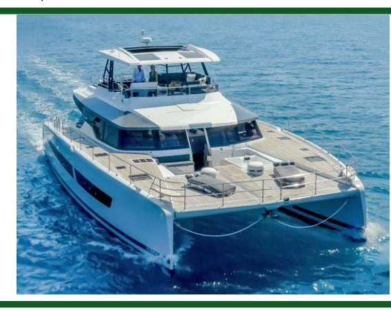
Type Modern Propulsion Power Hull Catamaran Length 19.5m (64') Beam 9.8m (33') Draft 1.2m (4') **Hull Material Fiberglass** 2 / Volvo / D6-480 Engine
